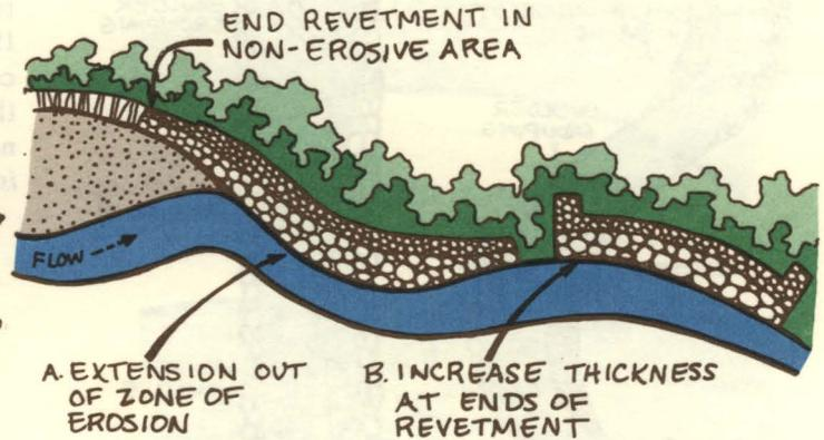
PLAN VIEW OF REVETMENT CONFIGURATION
