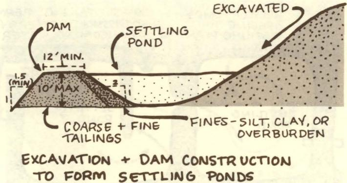
effective. The settling pond outlet should be wide enough to allow the top clear water to skim off while maintaining a low horizontal velocity.
