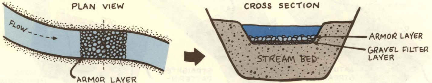
**Bank Stability:** Channel banks can be protected from erosion by revetment. Revetment will prevent lateral movement of the channel, but will also prevent plant regrowth, so use it only where necessary to stabilize the bank. Riprap of rubble or quarry stone is generally the most reliable and economical revetment.
