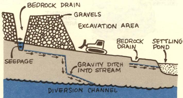
**Bedrock Drains:** Bedrock drains are used to collect groundwater that infiltrates the mine area. Two types of drains can be constructed: one that intercepts water above the mine area and diverts it into the stream or diversion channel, and one that collects water from within the work area and routes it to settling ponds.
