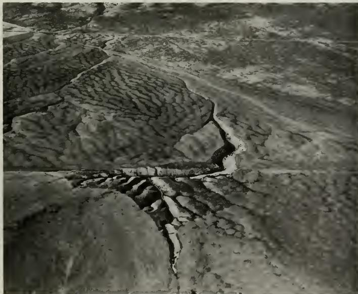
Photo 1. Aerial view southwest across low scarp of San Andreas fault exposed in the Carrizo Plain, Painted Rock quadrangle. Arroyos in Quaternary alluvial sediments shows 400 feet of right-lateral offset along fault.
