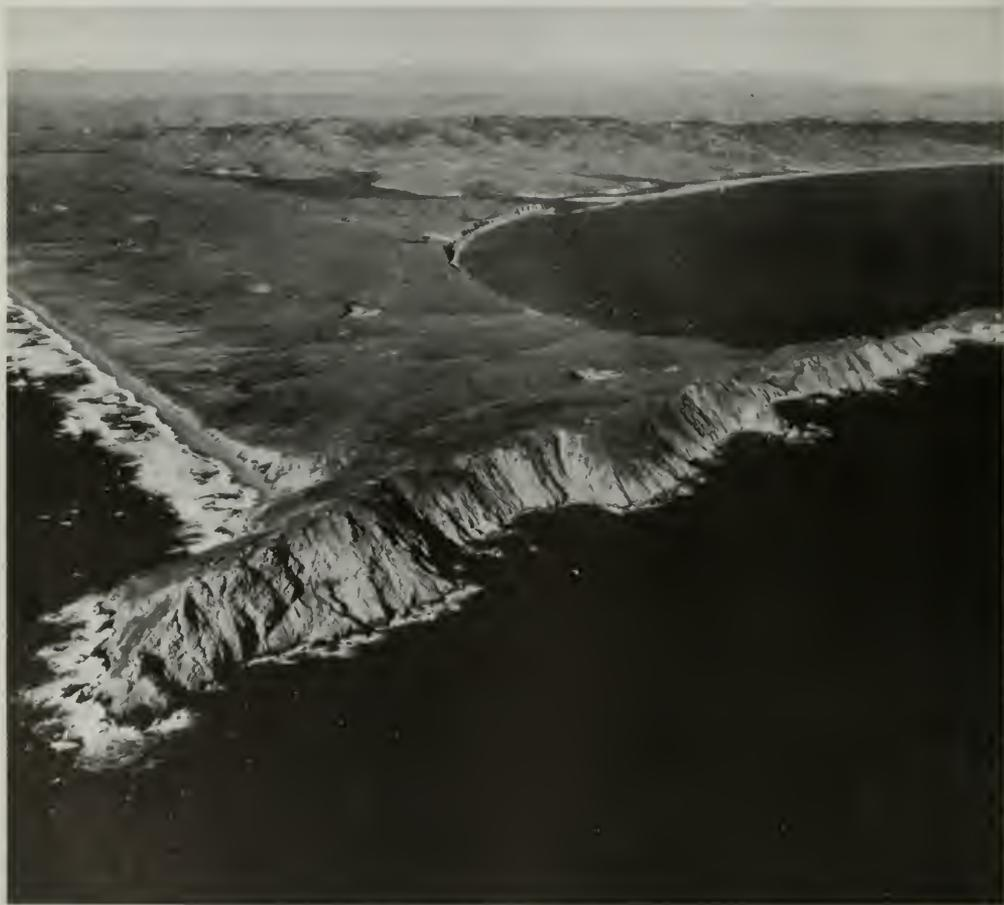
Photo 10. Aerial view north toward Point Reyes. On the left, perched near the water, can be seen the lighthouse. The bedded sedimentary rocks at the left (west) end of the Point are Paleocene conglomerates, which lie on Mesozoic granitic rock. In the middle distance, the Pliocene beds of Drake's Bay fill a syncline which is marked by the drowned valley of Drake's Estero. The San Andreas fault is just behind the first dark-colored distant ridge. Photo courtesy Aera Photographers, Sausalito.
