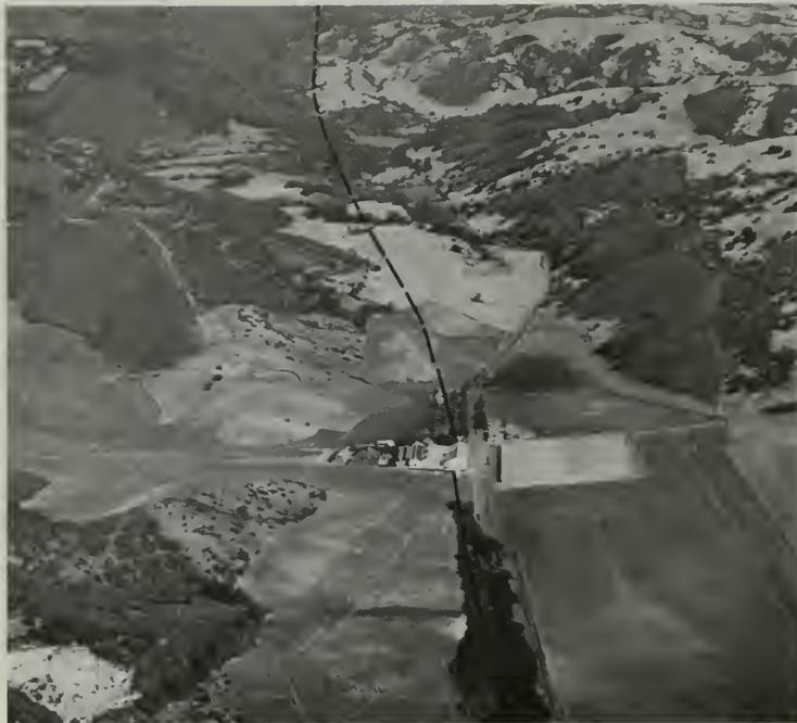
Photo 10. Aerial view of fault trace where it passes under Almaden winery south of Hollister. Line is approximate trace of fault. Looking northwest.
